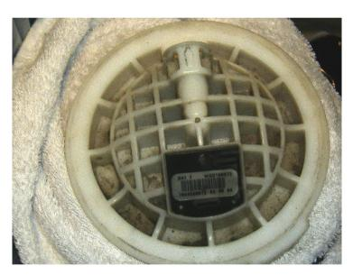
If your filter unit looks different, with two loops on top for lifting it out, you have the earlier filter. This kit is not applicable and you should not proceed further.
